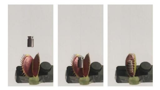
A new robotic grabber is ripped straight from the plant world. The device, made with a <u>Venus flytrap</u>, can grasp tiny, delicate objects.
